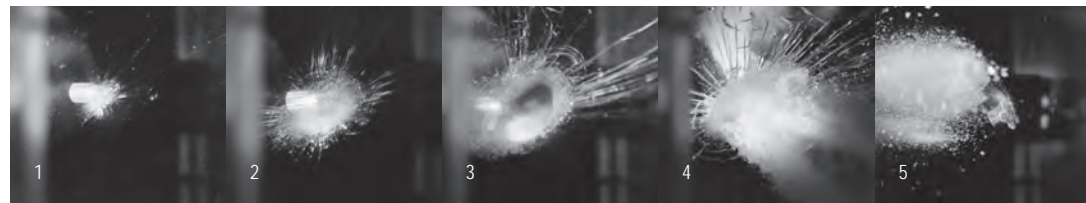
Sequence of high-speed photography showing the superior performance of Golden Saber HPJ Bonded through auto glass. Shot was set up to mimic one taken from the left front quarter of a vehicle. Frame 1: 230-gr., 45 caliber Golden Saber® Bonded bullet impacts typical windshield glass. Frames 2-4: Bullet passes through windshield. Frame 5: Emerges from the glass intact. Jacket and core held together through ASI ¼-inch laminated safety glass.
